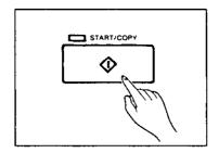
Press the START/COPY button to receive documents during a telephone conversation, and then place the handset on the cradle.
